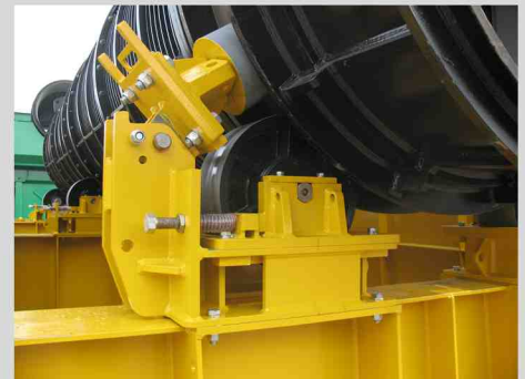
Drive, Support and Thrust rollers are easily accessible through the cassette base. Which can be easily removed if necessary
