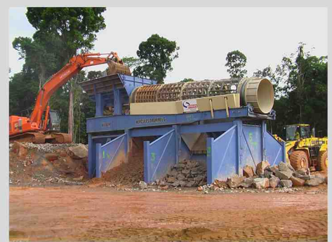
Skid frame for mounting the machine on. Reduces the cost of foundations as it eliminates concrete walls. Standard with the mobile machine.
