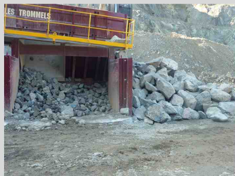
Optional chutes. Two chutes splitting one barrel to two sides of the machine giving two products. One chute from one barrel ideal for feeding onto a stockpile conveyor.
