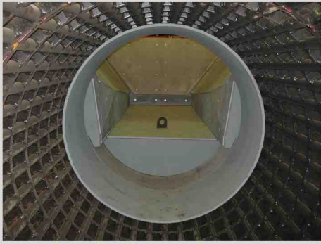
Heavy duty Feed Hopper stiffened with plate & sections. Tapered feed opening giving unrestricted transition from Feeder to Barrel.
